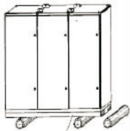
Rolling wood transportation (for transportation unit with weight < 1200kg)
